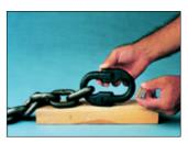
Place the locking sleeve between the assembled half link forgings.
