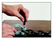
Place chain link into clevis of chain coupler. Insert pin fully into the clevis ears.
