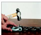
Place the coupler link on its side and using a hammer, drive the locking pin into the clevis ear until it is flush with the outside surface.
