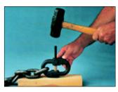
Drive the pin through the assembled link ends and sleeve until the end of the pin is flush with the outside of the connecting link halves.
