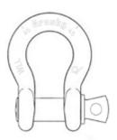
**SCREW PIN** Use when picking and placing a load, tighten pin prior to each lift.
