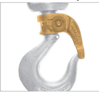
**To Lock:** Close the gate; a stainless steel pin is mounted in a horizontal bore which passes through the gate and engages a notch milled in the hook shank.
