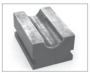
Never use dies that are cracked, worn or abraided (galled).
